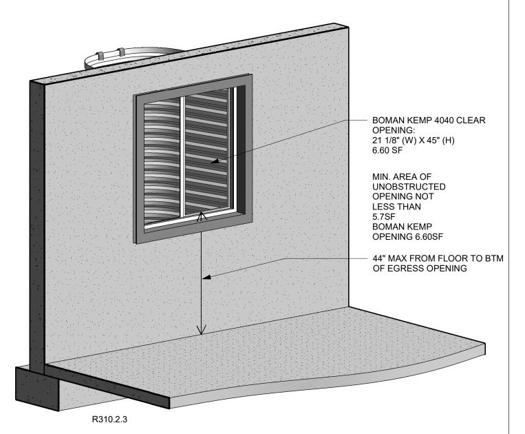
EMERGENCY ESCAPE AND RESCUE OPENINGS SHALL HAVE THE BOTTOM OF THE CLEAR OPENING NOT GREATER THAN 44 INCHES ABOVE THE FLOOR.
